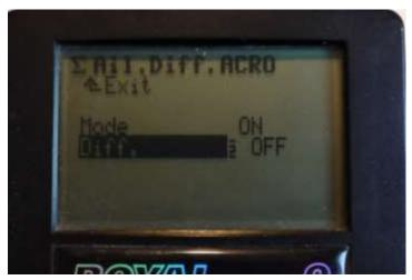
In flight phase 3 ACRO, 30% differential has been introduced, note the mode is +Spoiler, which differential is suppressed when the spoilers are deployed, note that this setting is not flight phase specific and if set in one phase it will be common to all phases.
