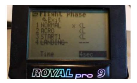
In the switch assignment menu, under setup (ABC1) the switch for phases 1-3 and main phase (flight phase 4) can be assigned
