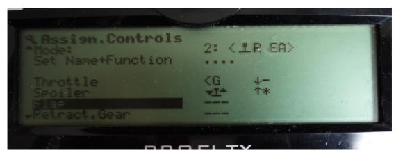
Spoilers assigned to stick and throttle to slider G, mode 2 so stick is on left. Note no control assigned to flap as this is set by flight phase in controls menu
