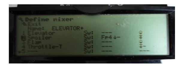
ELEVATOR + menu, this is the standard ELEVATOR + menu, note Elevator, Rudder, Flaps and Throttle - Trim inputs are always active, but spoiler input (for crow braking) is active on Fp4 only
