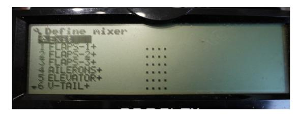
Mixer definitions are set up in the define mixer menu, which is in the setting menu, note this is the list of available mixer templates in the Glider+ model template which can cater for a glider wing with 8 separate control surfaces (4 per side), only FLAPS-1+, AILERON+ and ELEVATOR+ are used.
