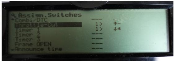
Throttle-cut and timer allocated to switch 1 on right hand side so that timer starts when throttle is active
