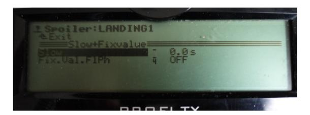
Note that while in this example we have made the spoiler input to the AILERONS+ and FLAPS-1+ mixers only active in Fp4 by assigning this as a switch, the same effect could be achieved by leaving the switch out of the mixer definition and setting a fixed value for flight phases where we don't want the spoiler control (stick) to work.
