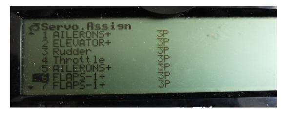
Servo assignment used, note if FLAP geometry on both flaps is significantly out and can't be matched with a 3 point curve then a 5 or 9 point calibration curve could be used
