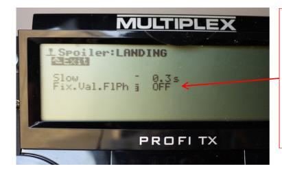
Here in flight phase 3, LANDING, the fixed input is OFF, this means that the spoiler control is active and the spoilers, if used, or any mixer that has spoilers as an input will respond to the spoiler control. Note also the slow setting, so if flight phase is switched and control is in fully deflected position, affected surfaces will only move slowly
