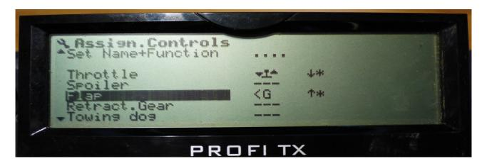
In the assign controls menu, select the required Flap control, here side slider G has been assigned, but they can be assigned to a 3 position switch if preferred
