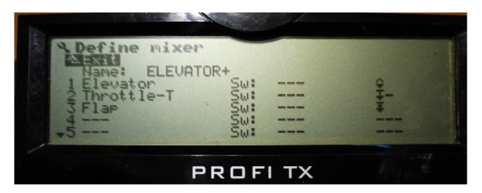
Select the ELEVATOR+ mixer and add Flap as one of the control inputs using the single side curve with two positions, the curves are covered in the mixer tutorial but this curve applies a mix which can be adjusted at the middle and end flap settings. Note other inputs are elevator, obviously, and also throttle without trim to allow some elevator compensation to be added if the model climbs or dives under power
