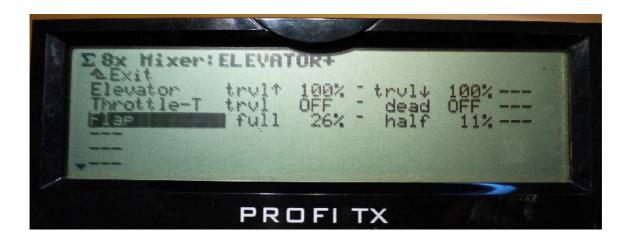
The Flap control input to the ELEVATOR+ servo can now be set at the mid and end position of the Flap control. Note if you find that the full position corresponds to the flaps in their up position and not fully down, you will need to enter the controls menu and reverse the action of the flap control by selecting the flap control and pushing the Rev/Clr button this will then change where the full mix has effect.
